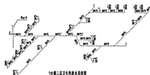
1#楼三层卫生间废水系统图 (1# Building 3rd Floor Bathroom Wastewater System Diagram)
