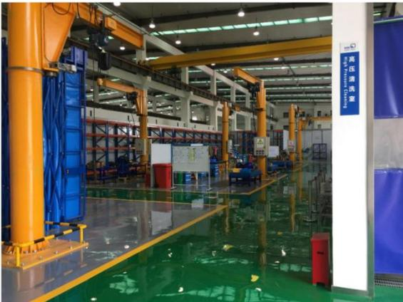
Guangzhou workshop covers an area of more than 1000 square meters, has a whole set of pump maintenance facilities, equipment and tools, with 5 tons of crane (can be expanded to 16 tons according to the circumstance in the future), the crane hoisting height 9 m. There are seven working stations, each of which is equipped with a one-ton cantilever. The cantilever is 3 meters long and hoisting height 4 meters.
