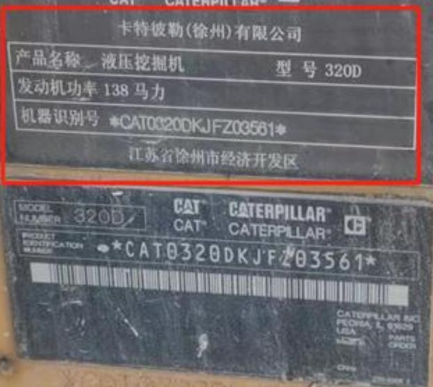
注: 1马力=0.7355KW, 功率: 138马力\*0.7355=101.4990KW
